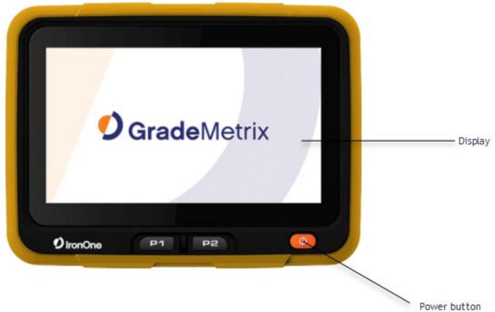
**Figure 1-1: IronOne front components**
