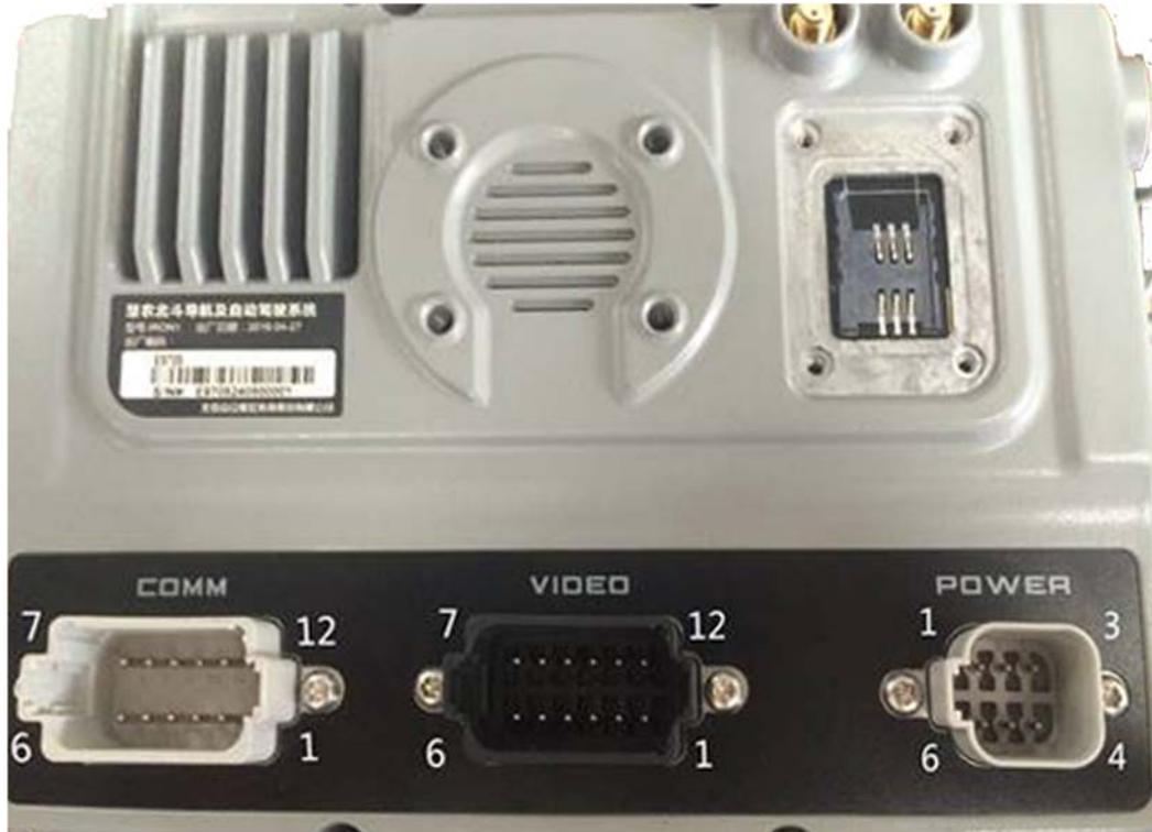
Figure 2-1: Display Pin-outs
